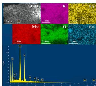
Fig.2 The EDS spectrum and mapping of the KLMO :0.80Eu<sup>3+</sup> phosphor.
