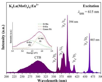
Fig.3 Excitation spectrum of the KLMO :0.80Eu<sup>3+</sup> ( $\lambda_{em} = 615$  nm).
