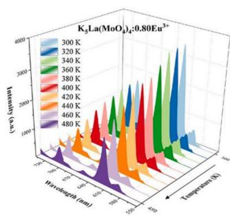
Fig.7 Three-dimensional PL spectra of KLMO:0.80Eu<sup>3+</sup> phosphor at different temperatures.
