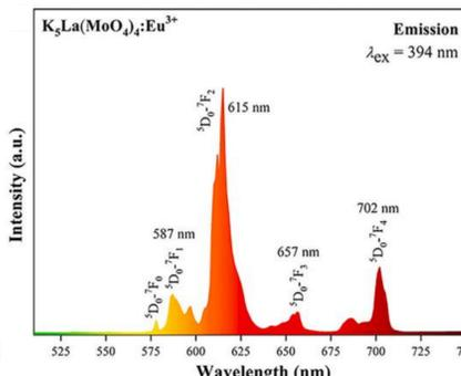
Fig.4 Emission spectrum of the KLMO :0.80Eu<sup>3+</sup> ( $\lambda_{ex} = 394$  nm).
