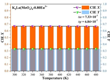
Fig.8 The temperature-dependent chromaticity coordinates of the KLMO:0.80Eu<sup>3+</sup>
