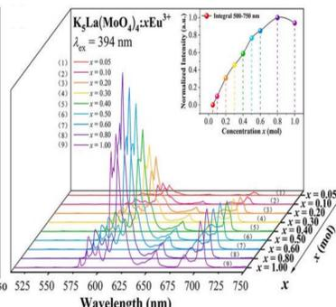
Fig.5 The PL spectra of KLMO:xEu<sup>3+</sup> (x = 5-100 mol%) phosphors with different concentration of Eu<sup>3+</sup> ions.
