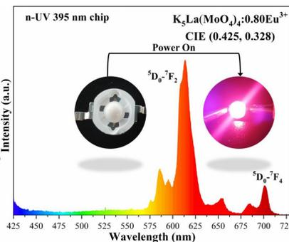
Fig.6 The EL spectrum of the red LED
