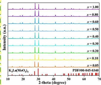
Fig.1 XRD patterns of the KLMO :0.80Eu<sup>3+</sup> samples.
